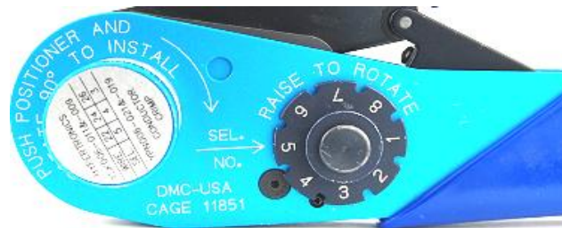
Fig. D. (Positioner inserted into Crimp Tool)
