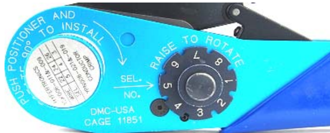
Fig. D. (Positioner inserted into Crimp Tool)
