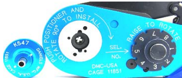
Detail A. (Positioner and Crimp Tool)
