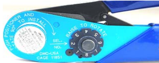
Fig. D. (Positioner inserted into Crimp Tool)
