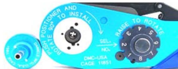
Detail A. (Positioner and Crimp Tool)
