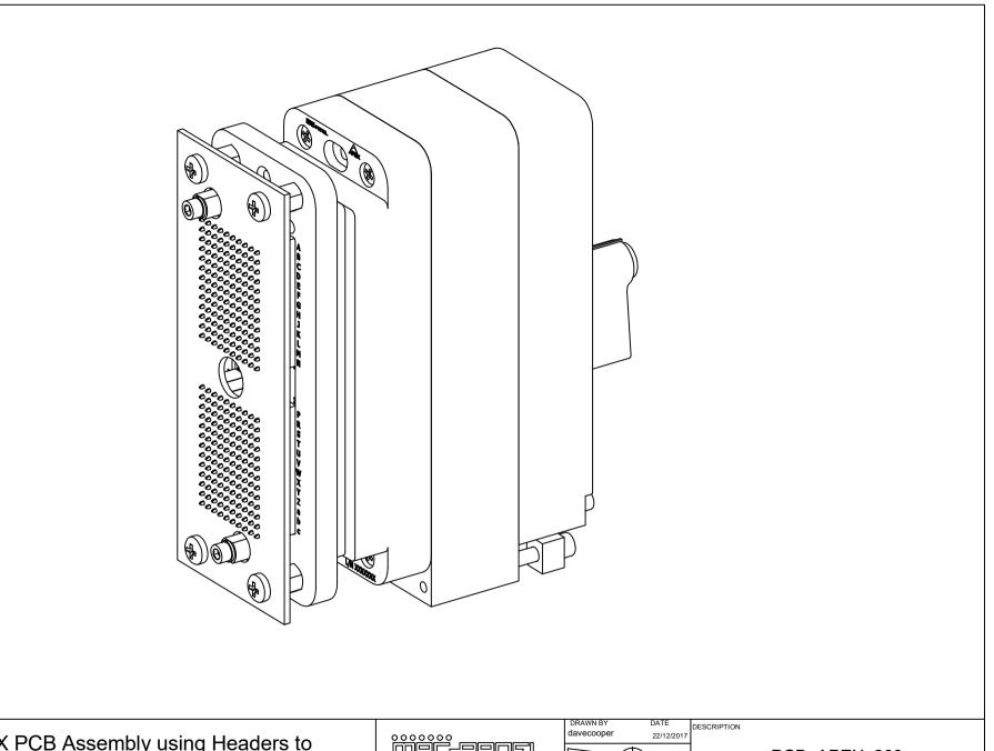
Example of an APEX PCB Assembly using Headers to enable simple Contact replacement.
